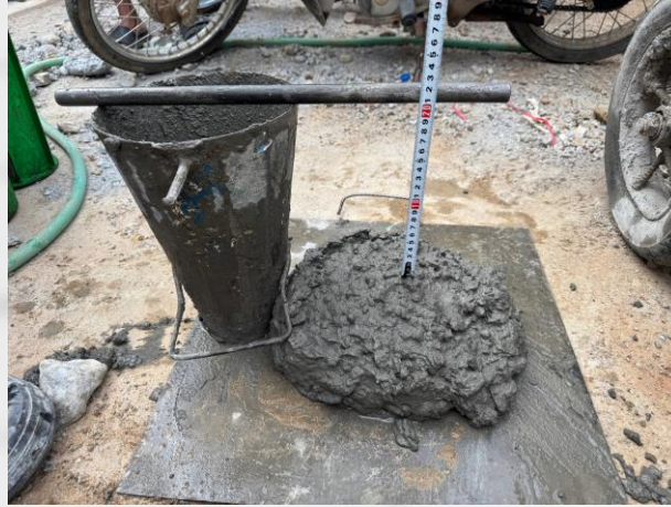
Slump Test: 21 cm.
